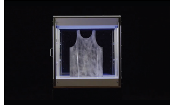
Figure 8: The prototype of the electroloom as presented in the paper of White et al. [14].
